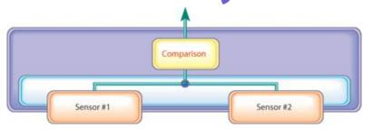
detect sensor failure with comparison (image source)
