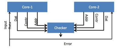
detect CPU fault with lockstep execution (image source)
